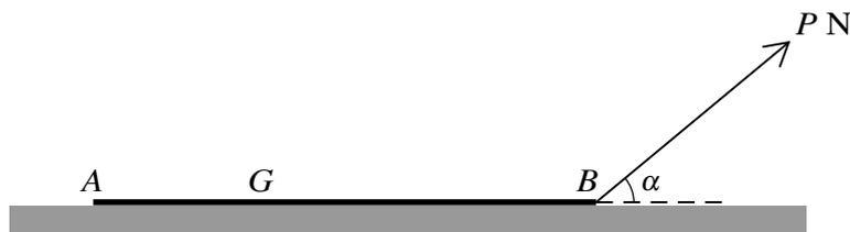
A non-uniform rod  $AB$  of mass 1.6 kg and length 1.25 m has its centre of mass at  $G$  where  $AG = 0.4$  m. The rod rests on a rough horizontal table. A force  $PN$  is applied at  $B$ , acting at an angle  $\alpha$  above the horizontal, such that the rod is in equilibrium but about to rotate about  $A$  (see diagram).
